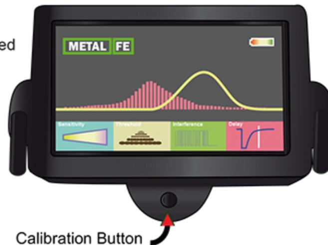
To enable the metal discrimination mode. With the coil level to the ground push the Calibration button, then sweep coil slowly from left to right for approximately 4 seconds.
