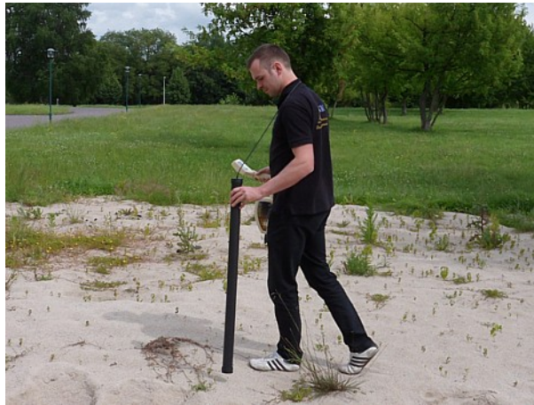
Figure 7.14: Position of the Supersensor during a measurement
