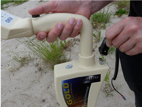
Figure 6.1: Connect control chip
