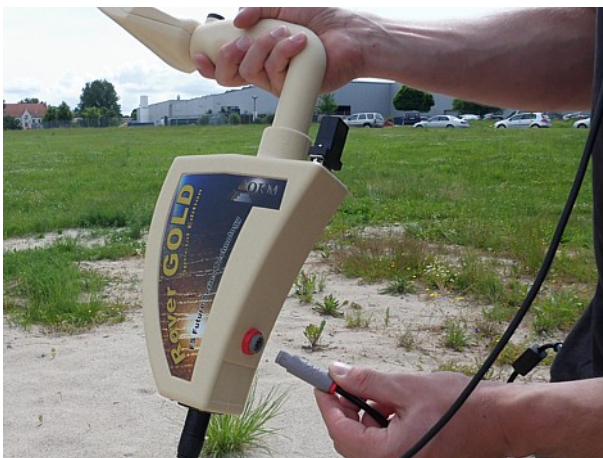
Figure 6.3: Connect power pack for power supply
