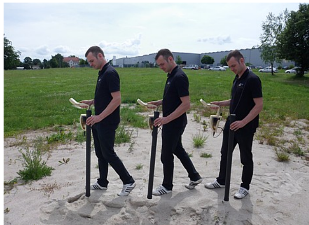
Figure 7.13: "Zig-Zag" scanning in mode Ground Scan
