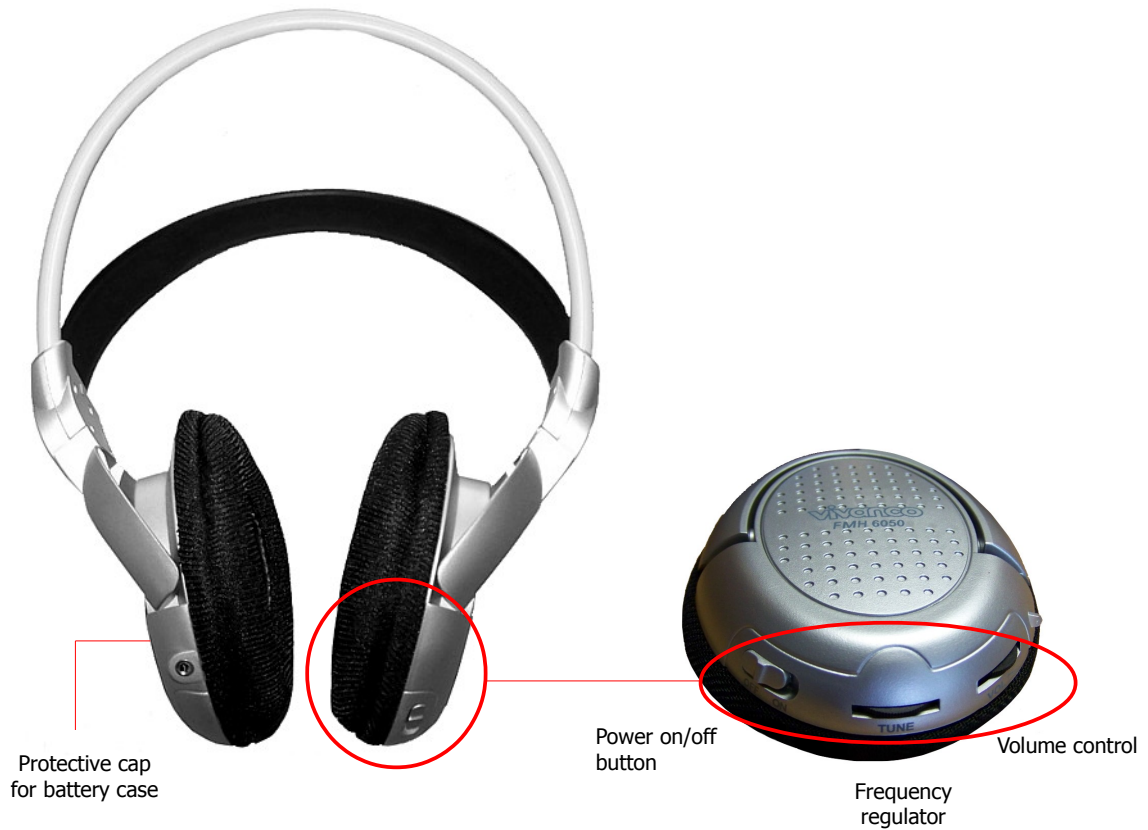
Figure 4.2: Control elements of wireless headphones
