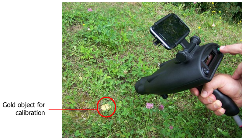
Figure 6.9: Calibrating the device onto a gold object in ionic mode
